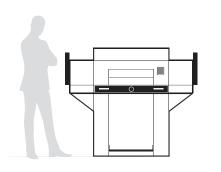
Dimensions 1370 x 1070 x 1400 mm (H x W x D) width with side tables 1630 mm
