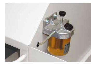
**EASY LUBRICATION** A centralised oiler for easy lubrication of the cutting head is standard equipment on this high-capacity shredder.
