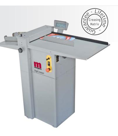
The DigiCreaser has a Head-up display for greater ease of use. This is particularly intuitive as it provides the operator with a series of prompts which are actioned by a single controller. These include positioning of the creases, setting the speed of the machine, storing jobs and counting facility.
