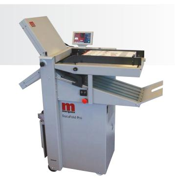
the fly if the fold plates or delivery roller needs to be moved. Within this SmartScreen panel are a counter and batching facility which are standard features. A further feature of the sophisticated SmartScreen is the ability to memorise and store repeated jobs in the alpha numeric memory which can then be retrieved within seconds.
